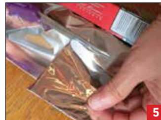
5 Cut out a small piece of aluminum foil big enough to cover the hole in the box. The best foil to use is a heavy-duty kind.
